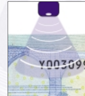
The sophisticated dual MG sensors detect the presence of magnetic ink, a common security feature among today's banknotes.
